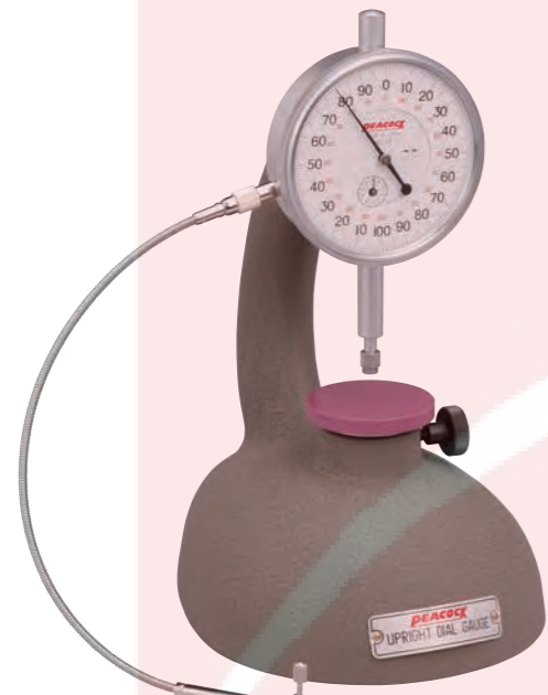
R1-A Graduation: 0.001mm Range: 2mm Effective measuring range: 10mm
