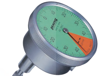
196Z Graduation: 0.01mm Range: 0.8mm ● Stem \phi 8mm ● Pointer giving less than one revolution ● Contact point (X-112)
