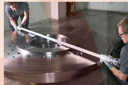
Radiused jaws for accurate ID measurement
